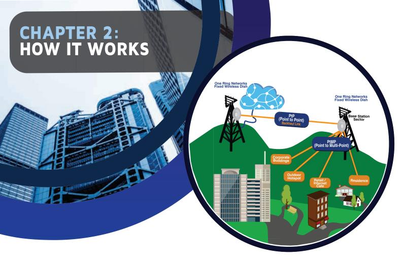
A fixed wireless radio transmitter is placed at the top of a tower, tall building, or mountaintop. These locations are called PoPs, meaning for Point of Presence. The elevated position provides the PoP with the perfect location to achieve a line of sight to buildings in the vicinity.
